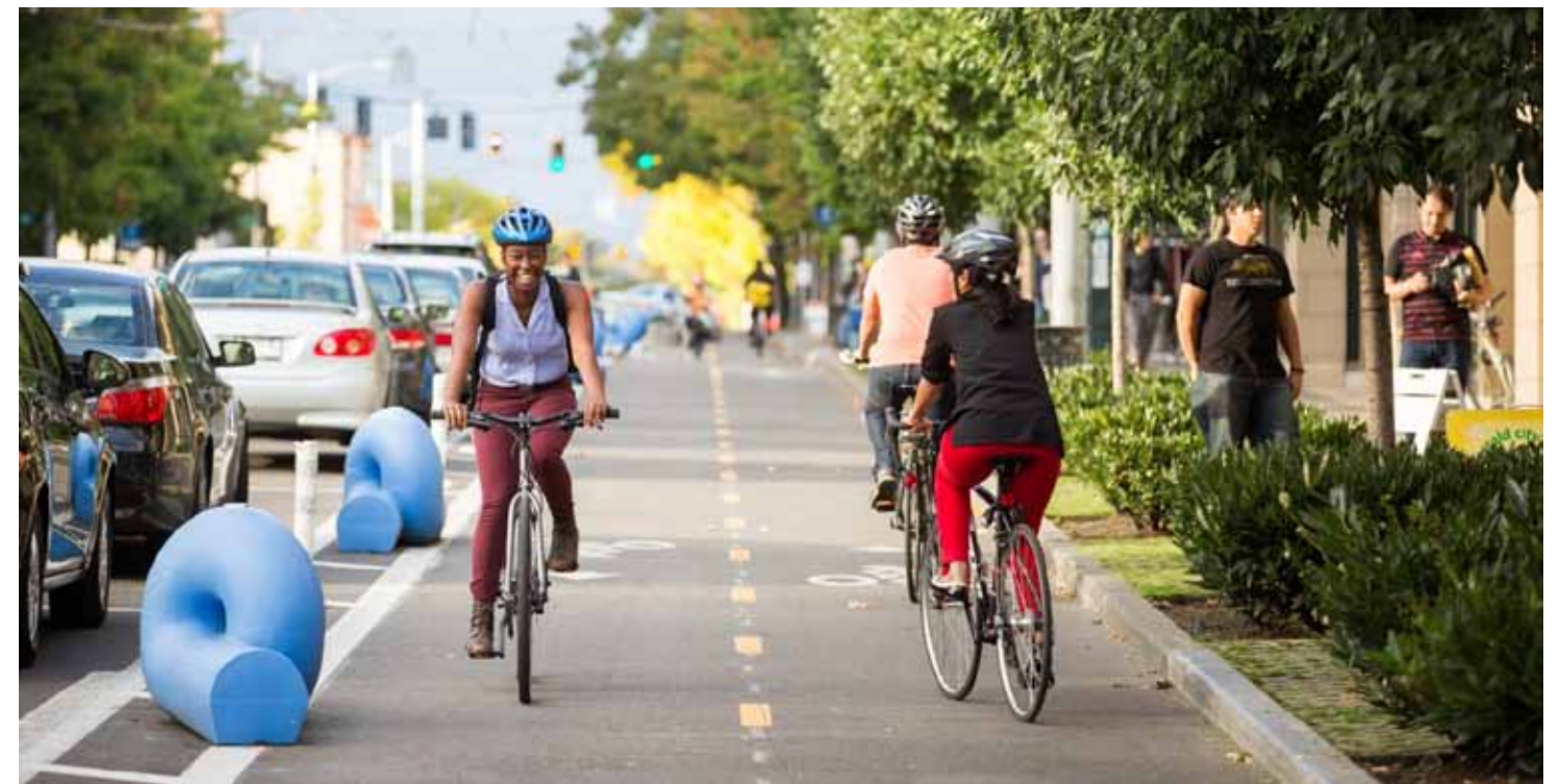
Broadway Bikeway, Seattle, WA Dedicated bike lanes that use sculptural pieces to separate bikes from vehicular traffic
